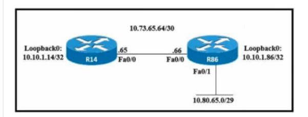
Refer to the exhibit. An engineer must configure a floating static route on an external EIGRP network. The destination subnet is the /29 on the LAN interface of R86. Which command must be executed on R14?
