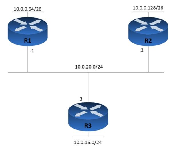
Refer to the exhibit. Router R1 is added to the network and configured with the 10.0.0.64/26 and 10.0.20.0/26 subnets. However, traffic destined for the LAN on
