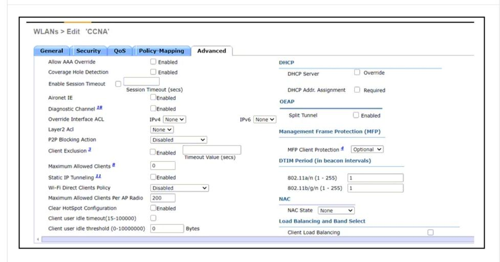
Refer to the exhibit. A network engineer configures the CCNA WLAN so that clients must reauthenticate hourly and to limit the number of simultaneous connections to the WLAN to 10. Which two actions complete this configuration? (Choose two.)
