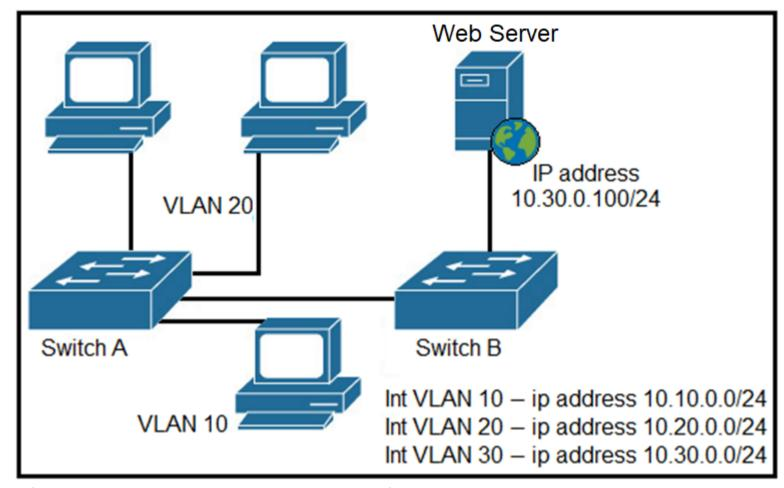
Refer to the exhibit. A network engineer must block access for all computers on VLAN 20 to the web server via HTTP. All other computers must be able to access the web server. Which configuration when applied to switch A accomplishes the task?
