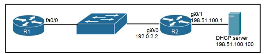
Refer to the exhibit. An engineer deploys a topology in which R1 obtains its IP configuration from DHCP. If the switch and DHCP server configurations are complete and correct, which two sets of commands must be configured on R1 and R2 to complete the task? (Choose two.)
