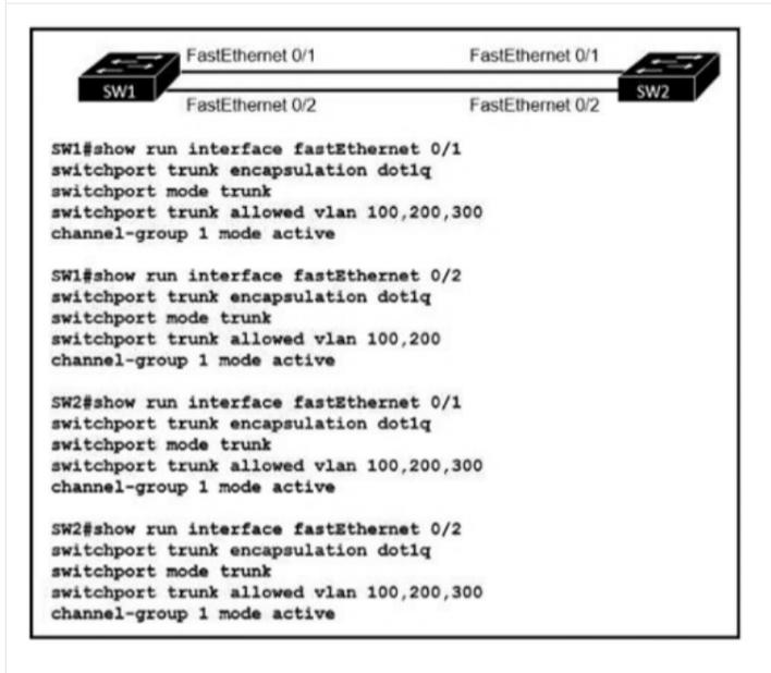
Refer to the exhibit. An engineer ts building a new Layer 2 LACP EtherChannel between SW1 and SW2, and they executed the given show commands to verify the work. Which additional task must be performed so that the switches successfully bundle the second member in the LACP port-channel?
