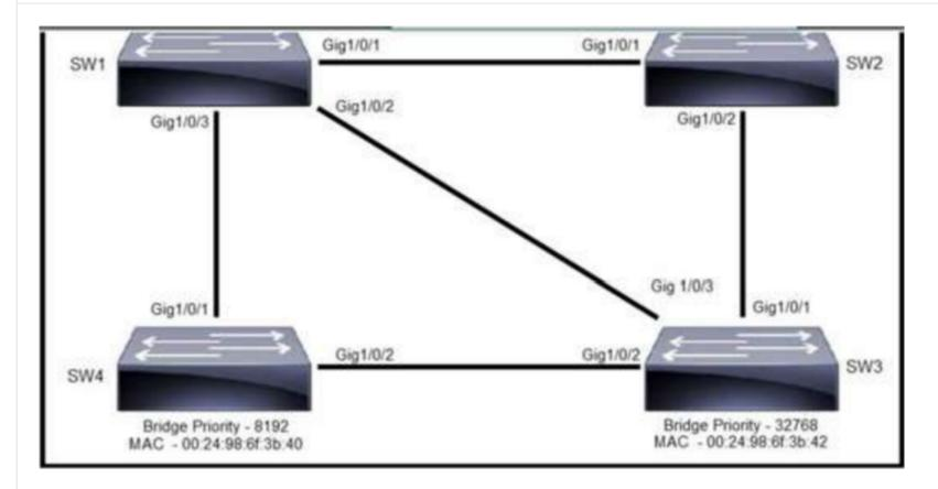
Refer to the exhibit. Rapid PVST+ mode is on the same VLAN on each switch. Which switch becomes the root bridge and why?
