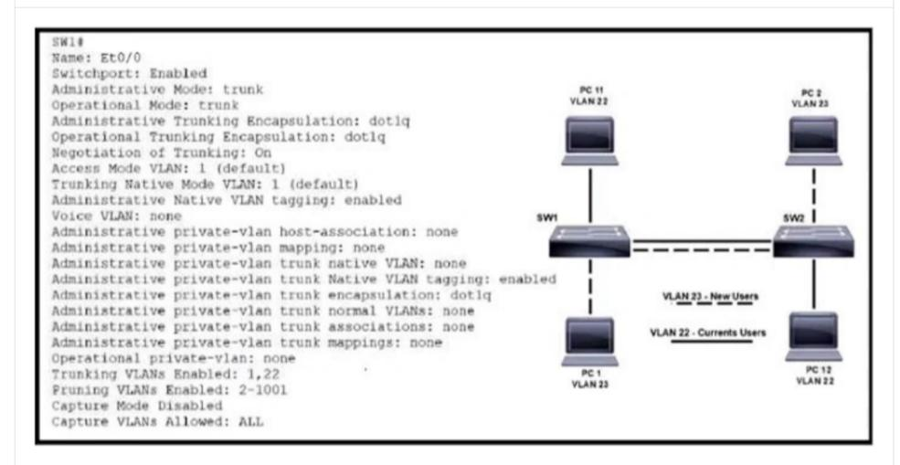
Refer to the exhibit. VLAN 23 is being implemented between SW1 and SW2. The command show interface ethernet0/0 switchport has been issued on SW1. Ethernet0/0 on SW1 is the uplink to SW2. Which command when entered on the uplink interface allows PC 1 and PC 2 to communicate without impact to the communication between PC 11 and PC 12?
