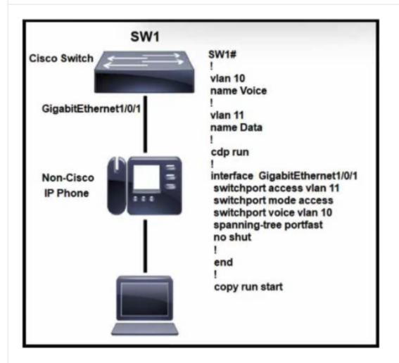
Refer to the exhibit. A multivendor network exists and the company is implementing VoIP over the network for the first time. Which configuration is needed to implement the neighbor discovery protocol on the interface and allow it to remain off for the remaining interfaces?
