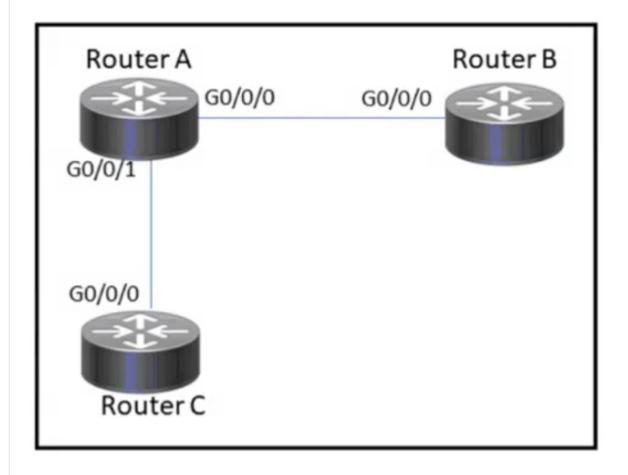
Refer to the exhibit. How must router A be configured so that it only sends Cisco Discovery Protocol information to router C?
