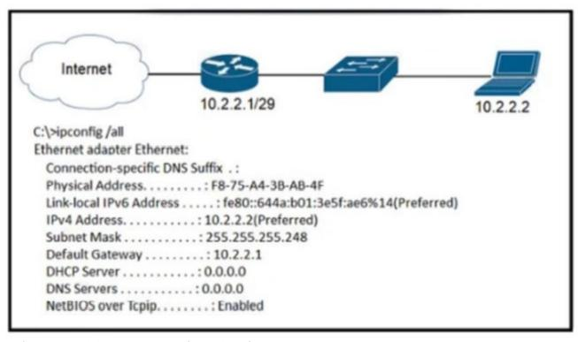
Refer to the exhibit. A newly configured PC fails to connect to the internet by using TCP port 80 to www.cisco.com. Which setting must be modified for the connection to work?
