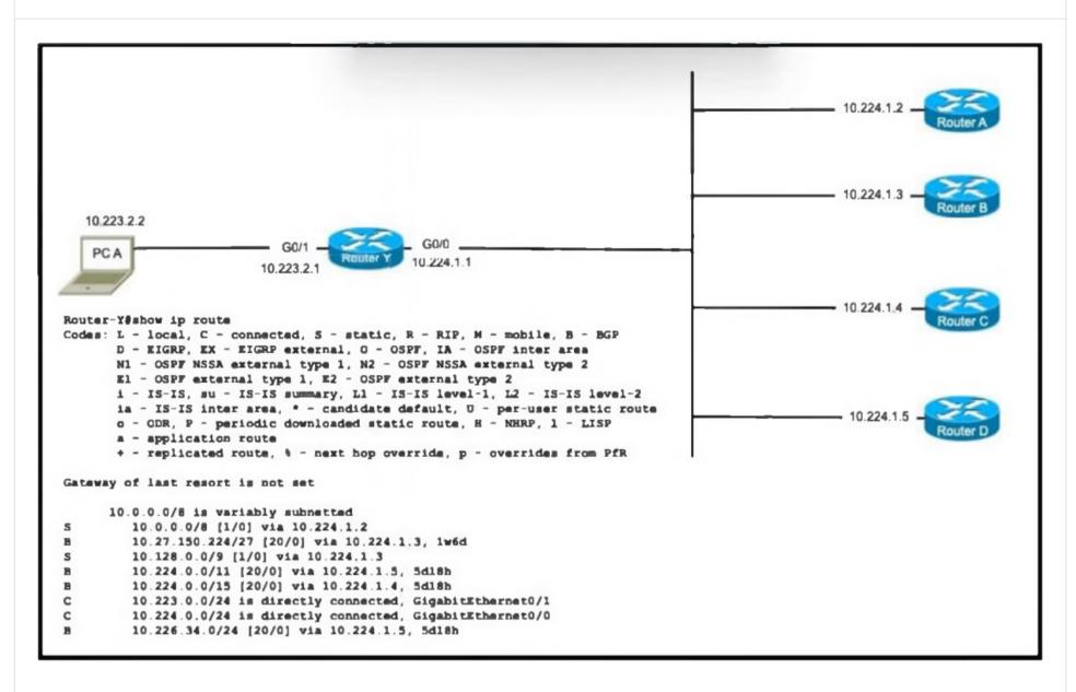
Refer to the exhibit. PC A is communicating with another device at IP address 10.227.225.255. Through which router does router Y route the traffic?
