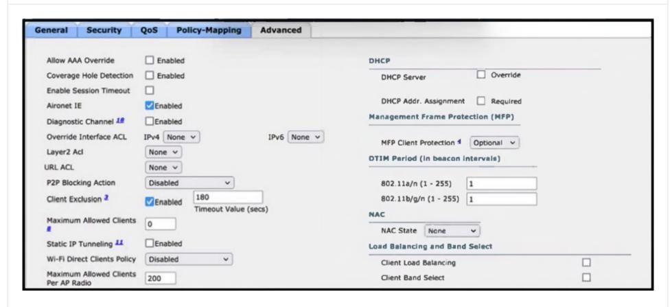
Refer to the exhibit. After a recent internal security audit, the network administrator decided to block all P2P-capable devices from the selected SSID. Which configuration setting must the administrator apply?
