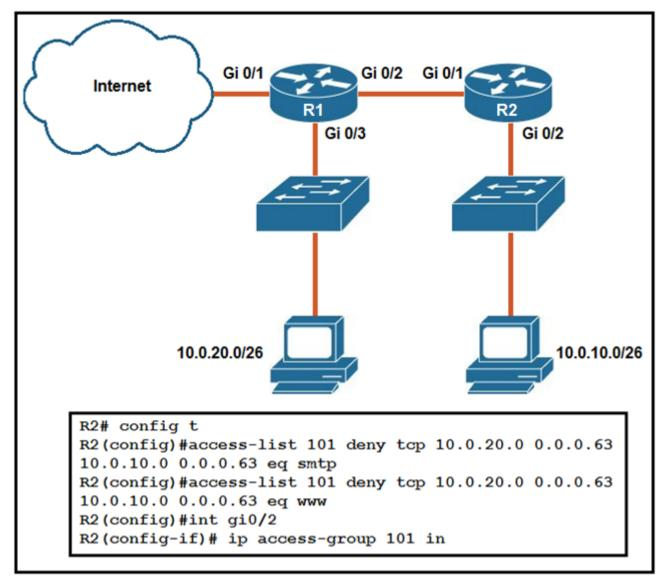
Refer to the exhibit. An extended ACL has been configured and applied to router R2. The configuration failed to work as intended. Which two changes stop outbound traffic on TCP ports 25 and 80 to 10.0.20.0/26 from the 10.0.10.0/26 subnet while still allowing all other traffic? (Choose two.)
