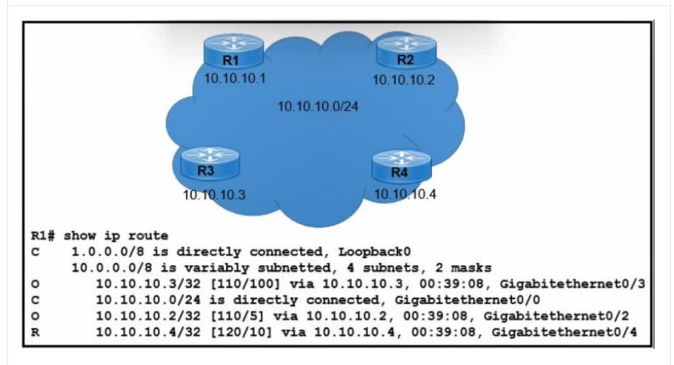
Refer to the exhibit. Which next-hop IP address has the least desirable metric when sourced from R1?
