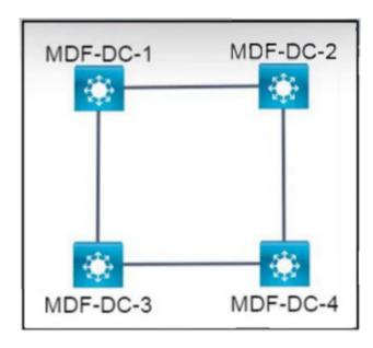
Refer to the exhibit. All interfaces are in the same VLAN. All switches are configured with the default STP priorities. During the STP elections, which switch becomes the root bridge?
