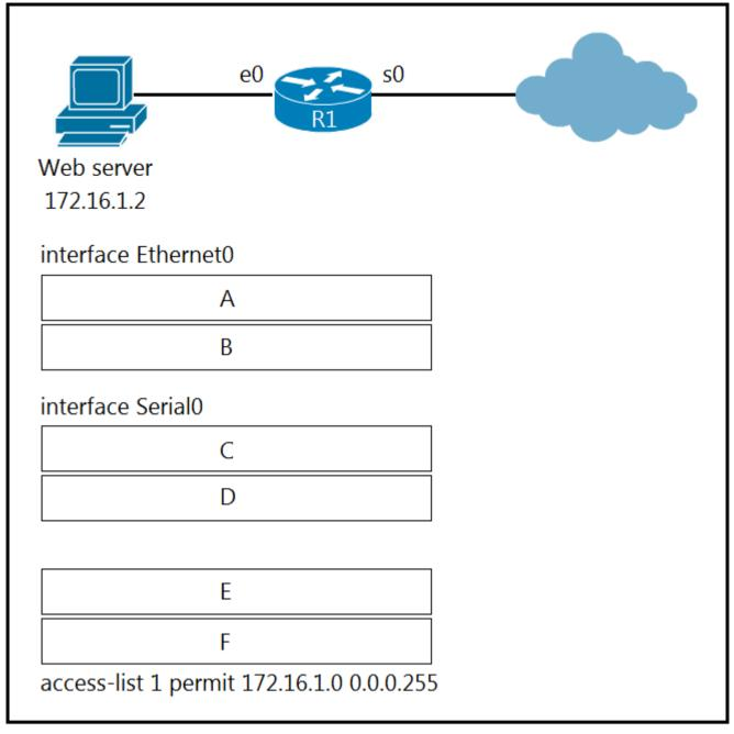
Refer to the exhibit. An engineer is configuring the router to provide static NAT for the webserver. Drag and drop the configuration commands from the left onto the letters that correspond to its position in the configuration on the fight.
