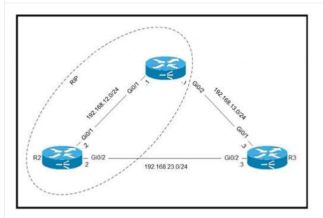
Refer to the exhibit. Routers R1 and R2 are configured with RIP as the dynamic routing protocol. A network engineer must configure R1 with a floating static route to service as a backup route to network 192.168.23. which command must the engineer configure on R1?
