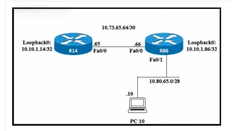
Refer to the exhibit. Router R14 is in the process of being configured. Which configuration must be used to establish a host route to a PC 10?
