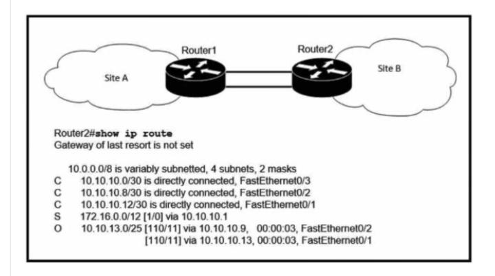
Refer to the exhibit. User traffic originating within site B is failing to reach an application hosted on IP address 192.168.0.10, which is located within site A. What is determined by the routing table?
