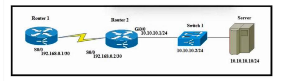
Refer to the exhibit. A network engineer must configure router R1 with a host route to the server. Which command must the engineer configure?
