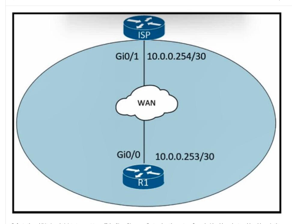
Refer to the exhibit. An administrator must turn off the Cisco Discovery Protocol on the port configured with address last usable address in the 10.0.0.0/30 subnet. Which command set meets the requirement?
