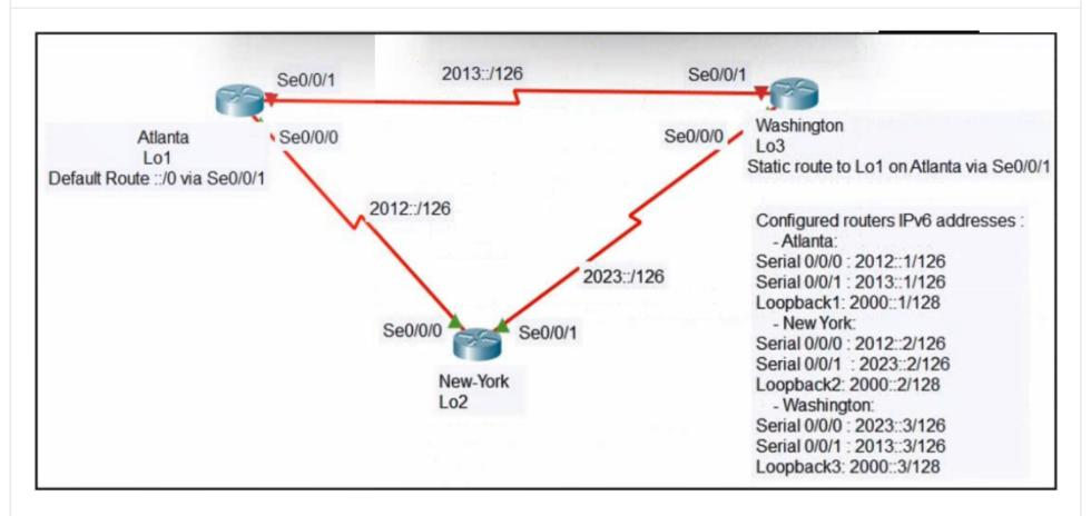
Refer to the exhibit. The New York router must be configured so that traffic to 2000::1 is sent primarily via the Atlanta site, with a secondary path via Washington that has an administrative distance of 2. Which two commands must be configured on the New York router? (Choose two.)
