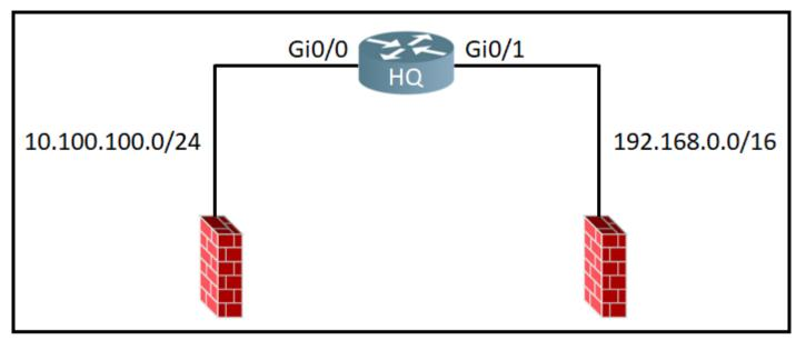
Refer to the exhibit. An access-list is required to permit traffic from any host on interface Gi0/0 and deny traffic from interface Gi0/1. Which access list must be applied?
