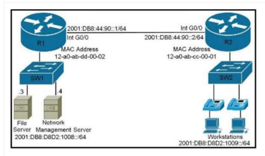
Refer to the exhibit. The iPv6 address for the LAN segment on router R2 must be configured using the EUI-64 format. Which address must be used?
