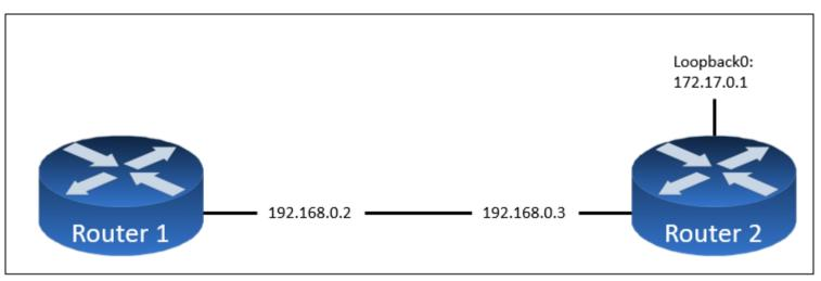
Refer to the exhibit. The ntp server 192.168.0.3 command has been configured on router 1 to make it an NTP client of router 2. Which command must be configured on router 2 so that it operates in server-only mode and relies only on its internal clock?
