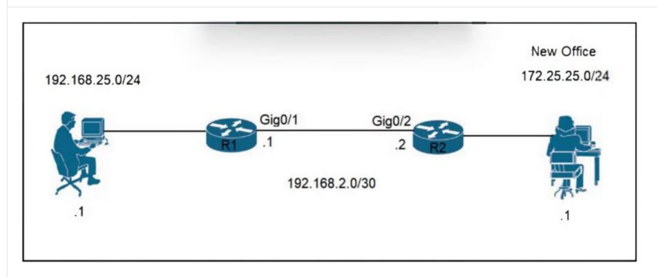
Refer to the exhibit. A network engineer is updating the configuration on router R1 to connect a new branch office to the company network. R2 has been configured correctly. Which command must the engineer configure so that devices at the new site communicate with the main office?
