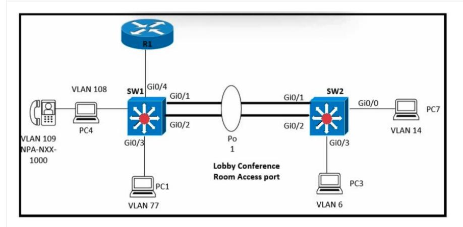
Refer to the exhibit. Which configuration enables an EtherChannel to form dynamically between SW1 and SW2 by using an industry-standard protocol, and to support full IP connectivity between all PCs?
