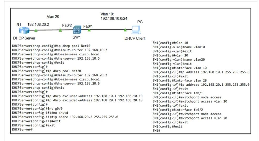
Refer to the exhibit. The DHCP server is configured with a DHCP pool for each of the subnets represented. Which command must be configured on switch SW1 to allow DHCP clients on VLAN 10 to receive dynamic IP addresses from the DHCP server?
