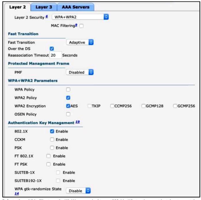
Refer to the exhibit. Clients on the WLAN are required to use 802.11r. What action must be taken to meet the requirement?
