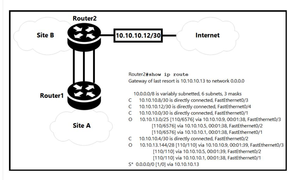
Refer to the exhibit. OSPF is running between site A and site B. Drag and drop the destination IPs from the left onto the network segments used to reach the destination on the right.
