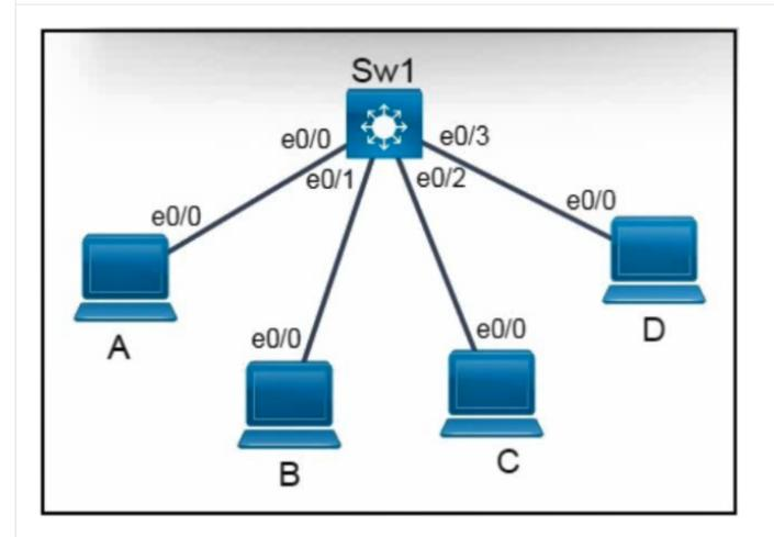
Refer to the exhibit. Host A switch interface is configured in VLAN 2. Host D sends a unicast packet destined for the IP address of host A.
