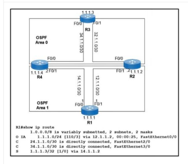
Refer to the exhibit. Which two values does router R1 use to identify valid routes for the R3 loopback address 1.1.1.3/32? (Choose two.)
