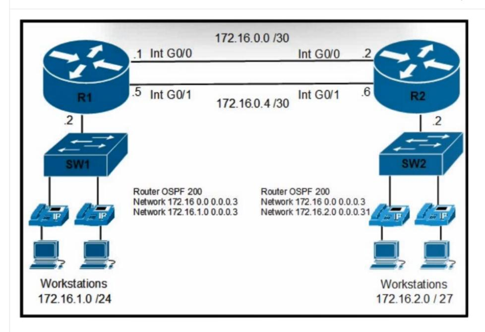
Refer to the exhibit. The primary route across Gi0/0 is configured on both routers. A secondary route must be configured to establish connectivity between the workstation networks. Which command set must be configured to complete this task?
